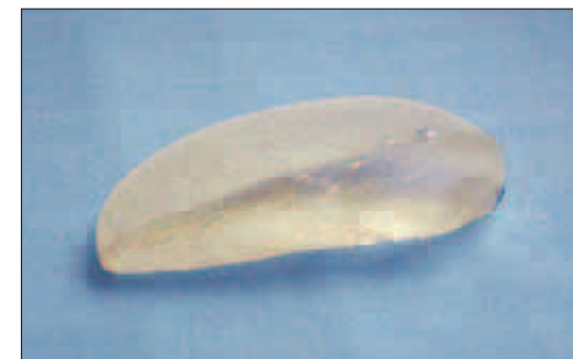
Photograph of a cohesive silicone gel implant cut in half - the silicone retains its shape due to increased cross-linking of the silicone molecules
